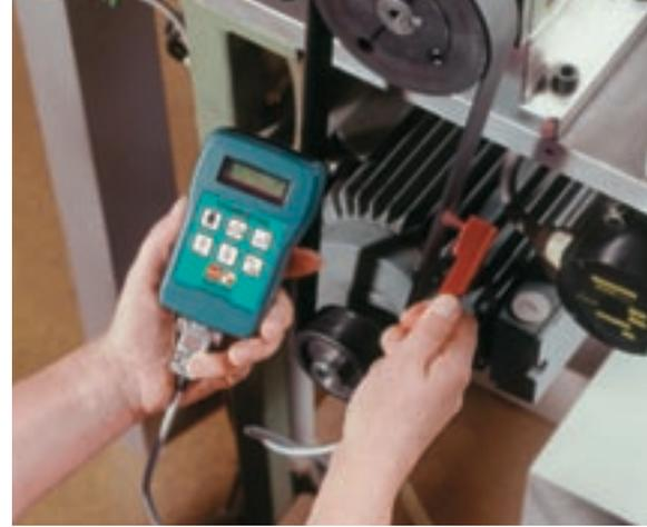
The distance between the drive belt and the measuring probe should be between 3 and 20 mm. See sketch for positioning.
