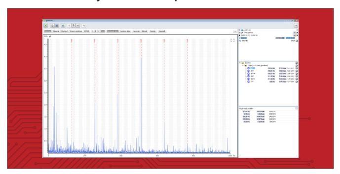
The SPM Spectrum measuring technique is a complement to the SPM dBm/dBc and LR/HR techniques. The purpose of SPM Spectrum is to verify the source of high shock pulse readings. Shocks generated by damaged bearings will typically have an occurrence pattern matching the ball pass frequency over the rotating race. Shocks from e.g. damaged gears have different patterns, while random shocks from disturbance sources normally do not coincide with the pattern of the machine element of interest.
