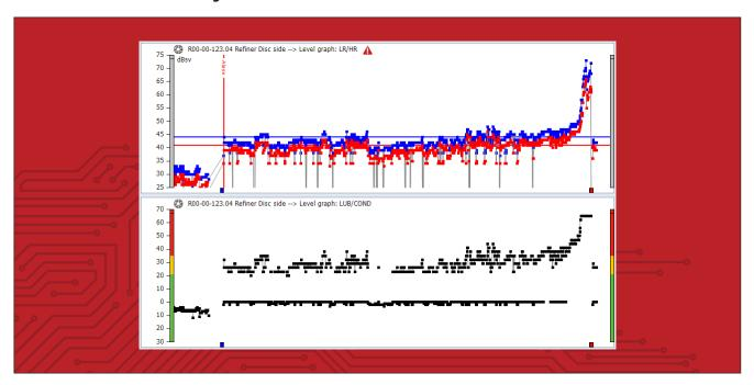
The LR/HR method was developed from the original Shock Pulse Method for condition diagnosis of rolling element bearings. It allows a precision analysis of oil film condition in the rolling interface and contains calculation models for finding the optimal lubricant. Poor lubrication is the root cause of most bearing failures.
