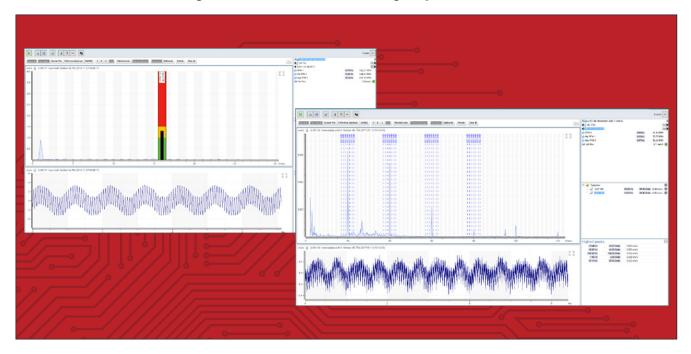
FFT Spectrum with symptoms is a vibration analysis function offered with Leonova and Intellinova. It is a reduced form of EVAM (see TD-591), lacking the statistical evaluation by means of criteria.
