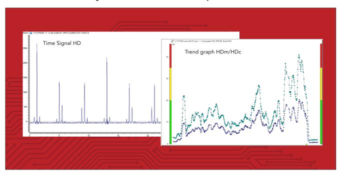
SPM HD Expert is a complement to SPM HDm/HDc and LR/HR. Advanced digital technique, RPM-based sampling frequency and measuring time automatically adjusted to RPM makes SPM HD particularly well suited for measurement on low speed applications. Extraordinary signal quality and 24 bit A/D conversion provides razor-sharp resolution and exceptional detail in spectrums and time signals.
