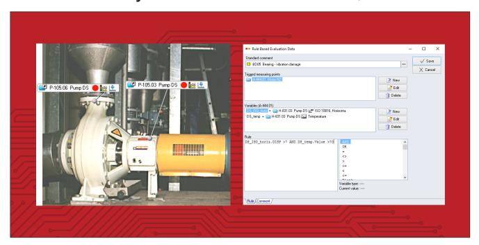
Rule-Based Evaluation (RBE) is a module in Condmaster Ruby. The purpose of RBE is to give the user guidance on what to do when certain alarm conditions are met. RBE is an excellent tool in Product Integrated Maintenance (PIM).
