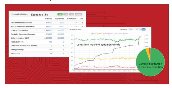
Plant Performer compiles and visualizes statistics relating to technical and economic KPIs (Key Performance Indicators) in the OEE/TEEP area for display and evaluation in Condmaster.NET. Plant Performer, a part of the Condmaster Ruby platform (see TD-583), demonstrates the benefits of condition monitoring and communicates its technical and economic impact to all levels of the organization.
