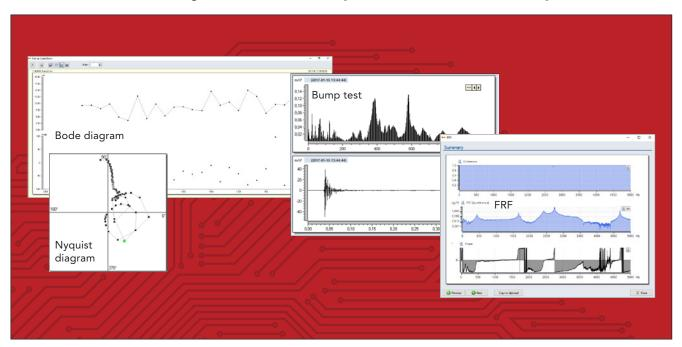
Run up/coast down measurements, Bump test and FRF are vibration analysis functions offered as a module for Leonova and Intellinova.
