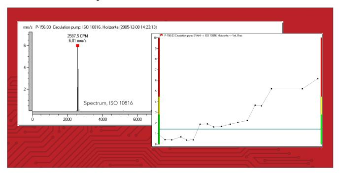
Broadband vibration measurement is the most widely used and cost-efficient method for the diagnosis of general machine condition.
