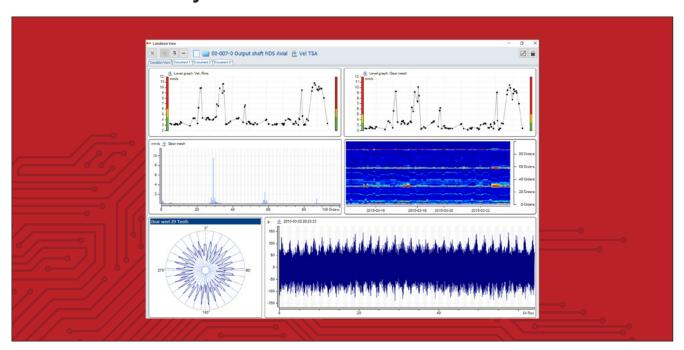
Condition View is a flexible and powerful function that makes it possible to combine multiple graphs in Condmaster into a single window for presentation and further analysis. The function can be used to show current machine condition, recent condition development or maintenance actions, e.g. to clarify or justify planned maintenance activities.
