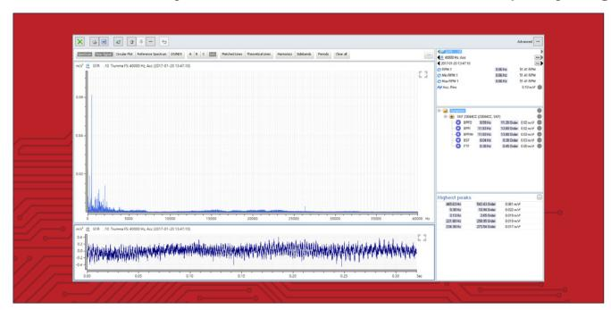
When higher resolution and frequency range are required for FFT with symptoms, EVAM, SPM HD Expert or SPM Spectrum, e.g. when monitoring high-speed gearboxes in turbines, MOD194 extends the maximum of these parameters. The lower frequency limit is then 0, 0.5, 2, 10 or 100 Hz. The upper limit is 40 000 Hz. The number of spectrum lines can be extended to max. 12 800 or 25 600.
