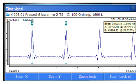
Gear symptoms SPM HD time signal
