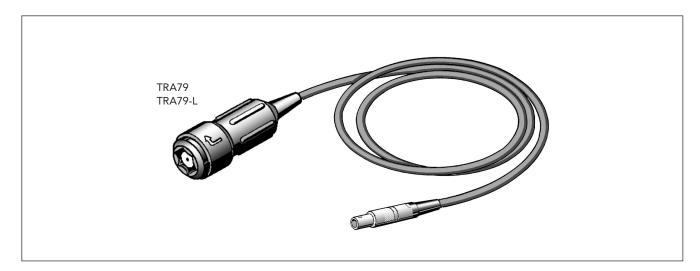
TRA79 is a shock pulse transducer with quick connector, used together with the handheld instrument Leonova Diamond<sup>®</sup> and Emerald<sup>®</sup>, for measurements on permanently installed adapters. The quick connector forms a bayonet connection together with the permanently installed adapter. Standard cable length is 1.5 m. Other lengths up to 20 m can be ordered.
