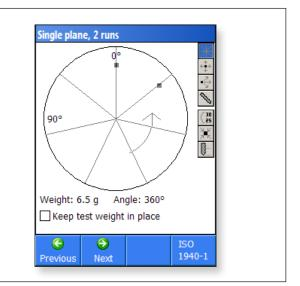
Leonova calculates a number of alternatives for correcting the unbalance:
