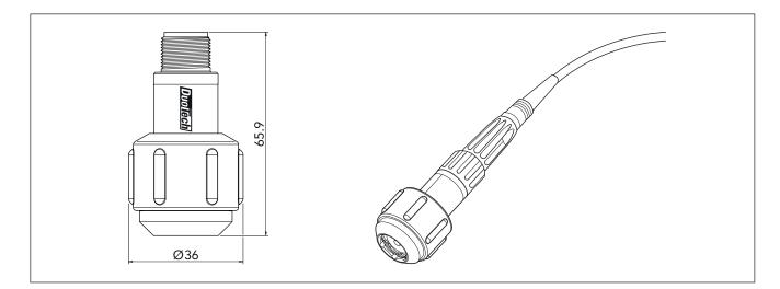
TRC150 is a DuoTech accelerometer with quick connector, used together with the handheld instrument Leonova Diamond and Emerald, for measurements on permanently installed adapters. The quick connector forms a bayonet connection together with the permanently installed adapter. The accelerometer is internally isolated in a Faraday shield providing maximum protection from ground loops and RF interference.
