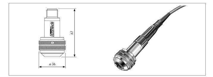
TRC100 is a DuoTech accelerometer with quick connector, used together with the handheld instrument Leonova Diamond and Emerald, for measurements on permanently installed adapters. The quick connector forms a bayonet connection together with the permanently installed adapter. The accelerometer is internally isolated in a Faraday shield providing maximum protection from ground loops and RF interference.
