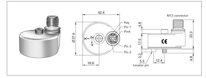
SPM 90546 is a low noise triaxial vibration transducer in rugged design with broad frequency response. It features a versatile M12 connector and an external case in a thick shell for high resistance to impact. Designed for both route-based and permanent-mount applications, this triaxial accelerometer hosts three general purpose, 100 mV/g vibration sensors with  $\pm$ 10% sensitivity tolerance. It has EMI/RFI and ESD protection.
