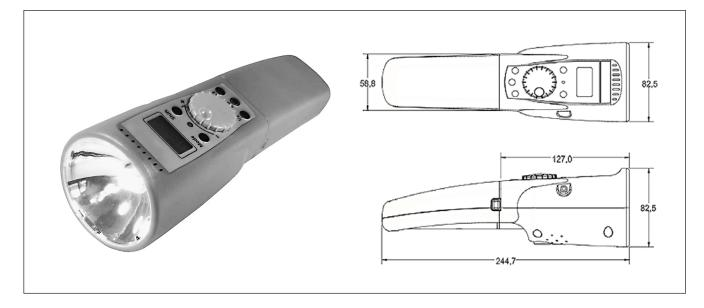
The Digital Hand Stroboscope 16936 is suitable for noncontact RPM measurements and for observation of fast, repeated motions of machines, their moving components or handled material from a distance of 20 to 50 cm.
