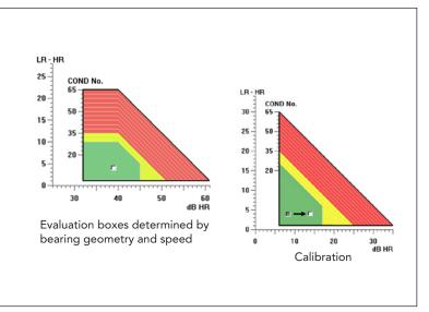
The LR/HR method was developed from the original Shock Pulse Method for condition diagnosis of rolling element bearings. It allows a precision analysis of oil film condition in the rolling interface and contains computation models for finding the optimal lubricant. Poor lubrication is the root cause of most bearing failures.
