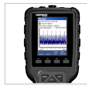
With Leonova, the HD ENV method is offered as an analysing function for unlimited use. It is a part of the packages Vibration Premium EME134 (TD-366) and Vibration Supreme EME193 (TD-445).
