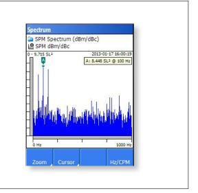
The purpose of SPM Spectrum is to verify the source of high shock pulse readings. Shocks generated by damaged bearings will typically have an occurrence pattern matching the ball pass frequency over the rotating race. Shocks from e. g. damaged gears have different patterns, while random shocks from disturbance sources have none.
