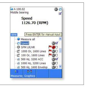
Recording is an Leonova function included in the platform. It allows the user to measure and record measuring results over longer periods of time, up to 50 hours. The recording function is an analysis tool which can show the interaction of various condition parameters over time.
