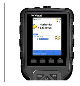
Broadband vibration measurement is the most widely used and cost-efficient method for the diagnosis of general machine condition. There are two ISO recommendations concerning this type of machine condition monitoring; the much used ISO 2372 and the more recent ISO 10816, which is a ongoing replacement of the older standard.
