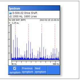
The method uses multiples of rotational speed (orders), rather than absolute frequency (Hz). The number of orders to be shown is input by the user. Leonova will then automatically set the sampling frequency to an exact multiple of the measured rpm. Order tracking will also minimize the risk of smearing when using FFT averaging.
