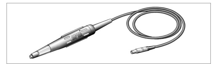
TRA78 is a handheld probe, used together with Leonova Diamond<sup>®</sup> and Emerald<sup>®</sup>. The probe is directionally sensitive and must be held aligned against the bearing and not deviate from this direction by more than  $\pm 5^{\circ}$ . The probe tip is spring loaded and moves within a sleeve made of chloroprene rubber (neoprene) and tolerates 110 °C (230 °F). Standard cable length is 1.5 m. Other lengths up to 20 m can be ordered.
