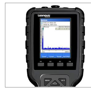
FFT Spectrum with Symptoms is a vibration analysis function offered with Leonova, part of EME134 or EME193.
