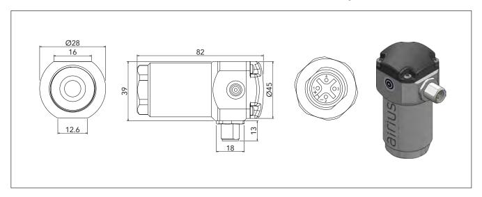
Airius is a wireless sensor that performs a user-defined number of vibration measurements per day in the 10-1000 Hz or the 2-1000/10-5000 Hz frequency range. The MEMS (micro-electro-mechanical-systems) type sensor with digital output measures triaxial vibration and temperature.
