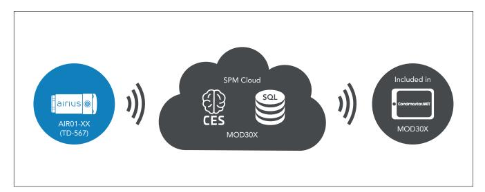
The SPM Cloud solution with monthly subscription enables access to measurement data from the Airius sensors. Stored in SPM Cloud, the smart data from CES (Condmaster Entity Server) can be viewed in Condmaster.NET from any device with Internet access – anytime, anywhere in the world.
