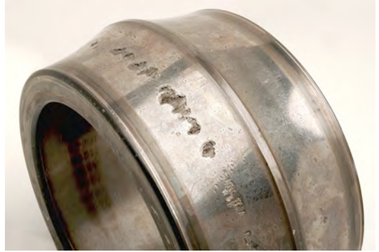
Above: Disassembled bearing with spallings.
